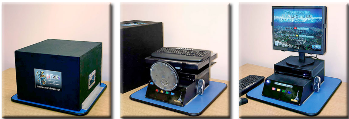
An example of a modular exhibit: the PP45S LHC simulator. Everything needed to run the unit is stored in the carrying case, which is an integral part of the base assembly.
